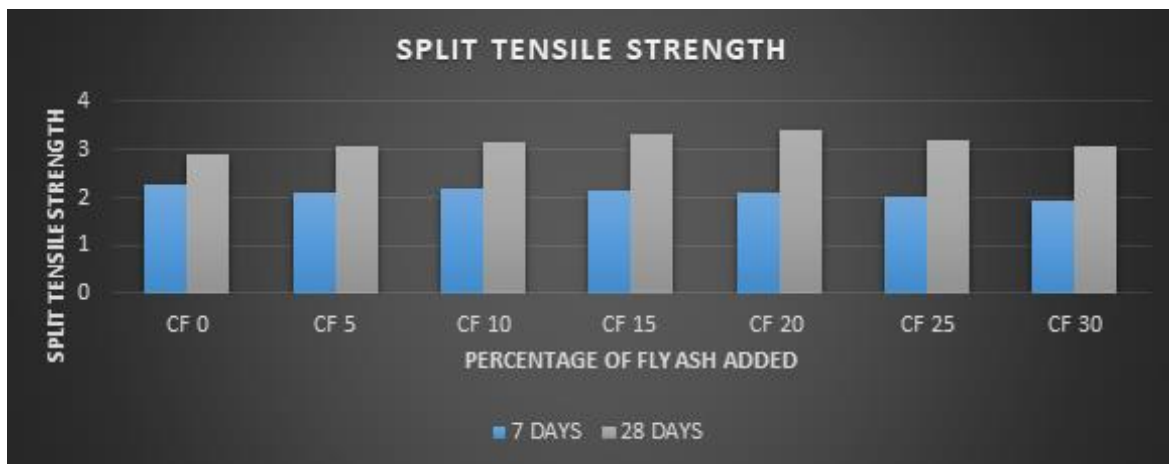
Fig: 5.9 split tensile strength with 10mm retained aggregate
