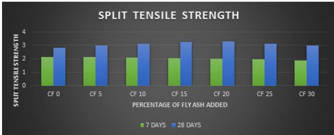
Fig:5.10 split tensile strength with 12.5mm retained aggregate
