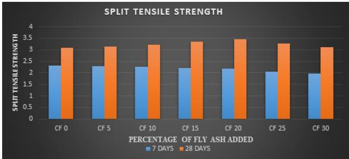
Fig:5.8 split tensile strength with 4.75mm retained aggregate
