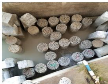
Figure 2: Curing of test specimens
