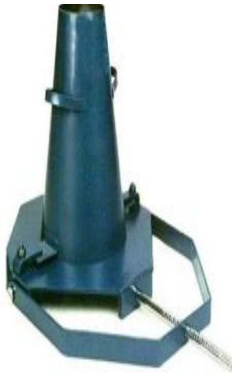
Figure 3: Slump cone arrangement
