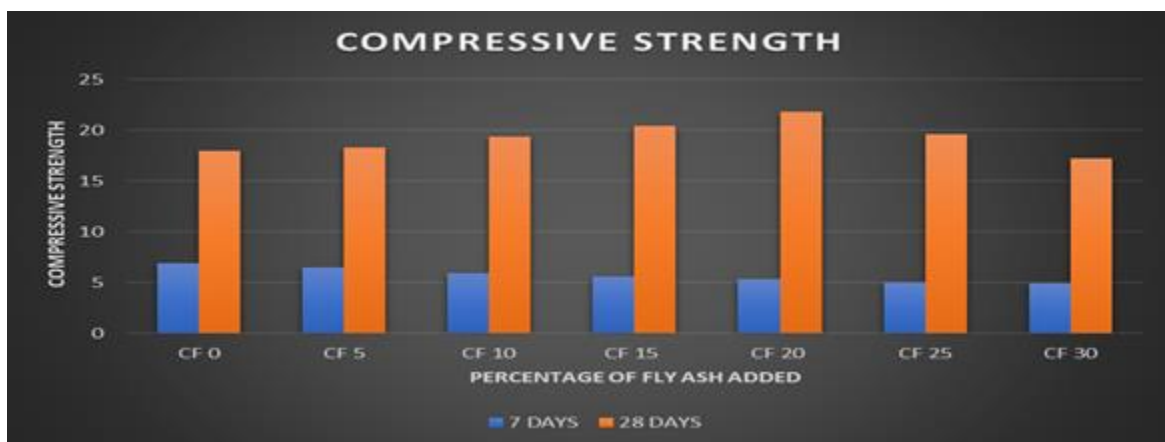
Fig:5.5 Compressive strength with 4.75mm retained aggregate
